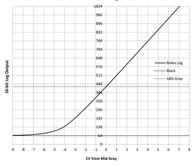
The Bolex Log transfer function covers a wide dynamic range to prevent clipping values that are captured by the D16. 18% gray is encoded at the code word 428/1023 and black level is fixed at 64/1023. The linear part of the above graph spans a 10 stop range and encodes the values with about 83 code words per stop in a 10-bit encoding.
