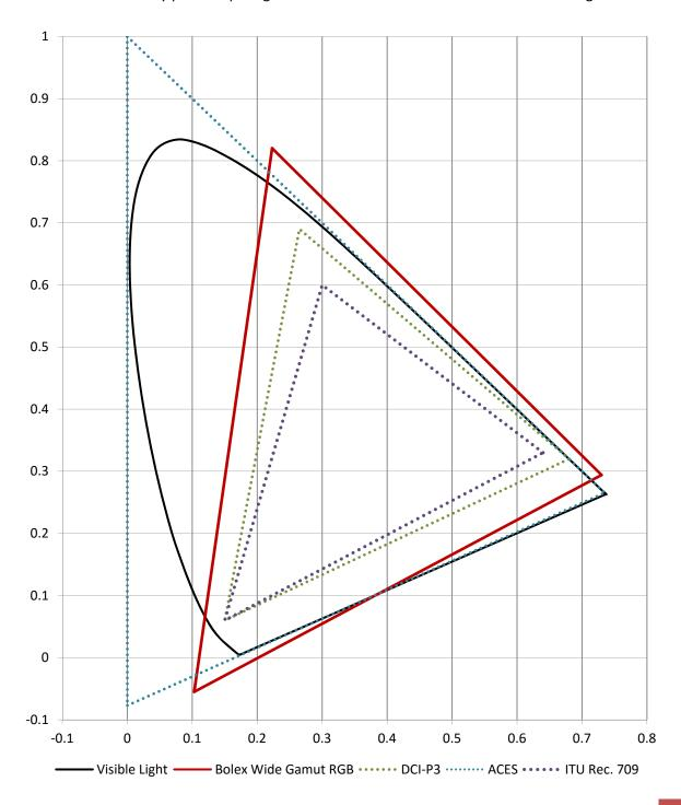
The following are the corresponding chromaticity values that create the vertices of the above color gamuts. Color matrices to convert between these color gamuts can be calculated from this table of values. Conversions must be applied only on linear footage. When converting Bolex Wide Gamut RGB to color gamuts with white points other than D65, it's recommended to use the Bradford transform for chromatic adaptation.
